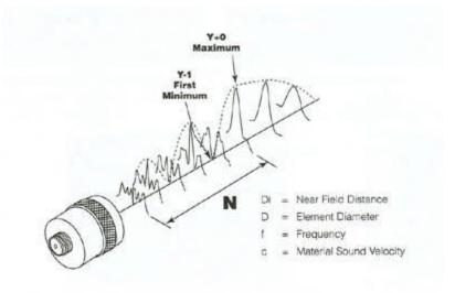
The sound field of a transducer has two distinct zones. These zones are called the near field, which is the region directly in front of the transducer, and the far field which is the area beyond "N" where the sound field pressure gradually drops to zero. Because of variations of the near field, it may be very difficult to accurately measure and evaluate flaws.
