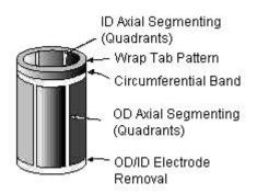
The field of fiber-optics research has benefited from the uniform radial expansion of the tube OD, to stretch optical fibers for enhanced signal tuning. Tube sizes can be custom fabricated to maximize radial expansion for this fiber optic application.
